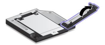
3. Lift up the cover film and insert the hard disk drive with the label facing upward.
